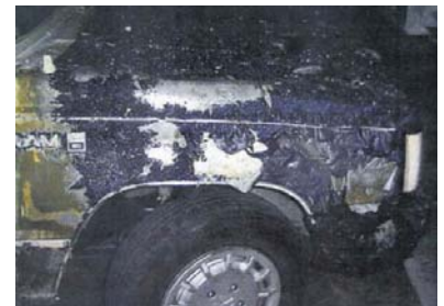
Bubbling paint ready for removal
